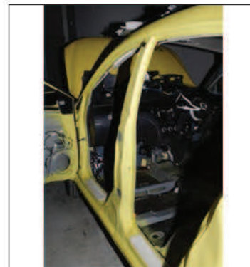
P3-21A: Maximum B-pillar intrusion 42mm
