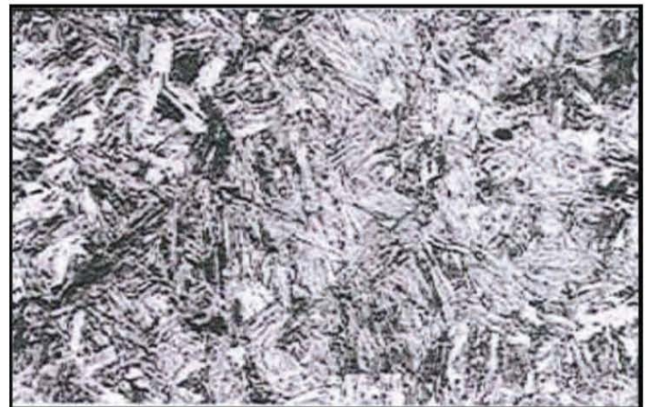
Figure 4: Metal microstructure after quenching martensite
