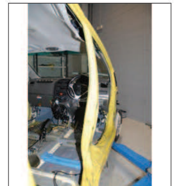
P6-20A: Maximum B-pillar intrusion 168mm
