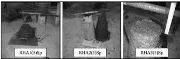
Figure 1: The slump for various mixes of fresh RHA concrete
