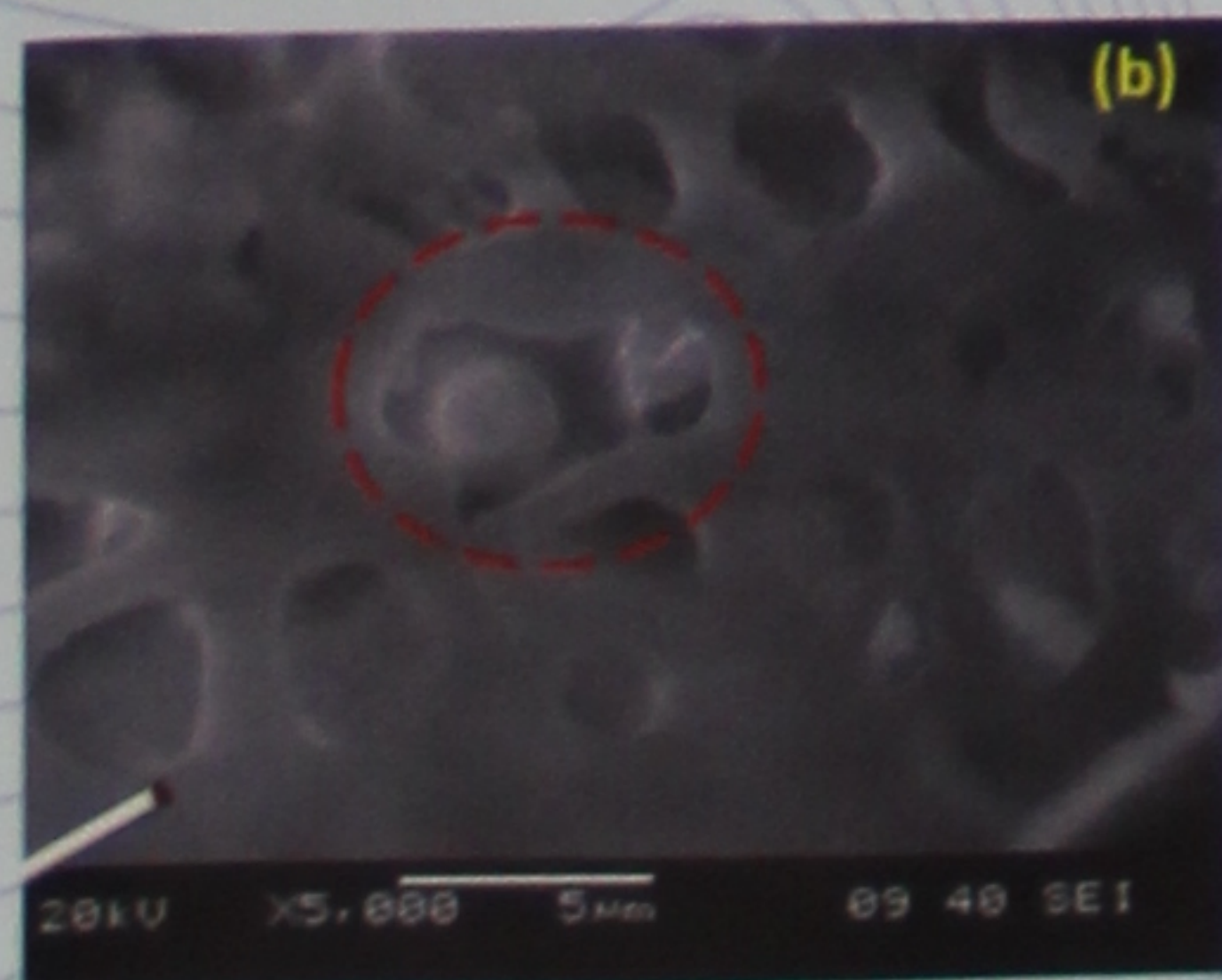
Figure 1: SEM images of Activated carbon fiber sheet (a) before and (b) after adsorbing the sidestream cigarette smoke.
