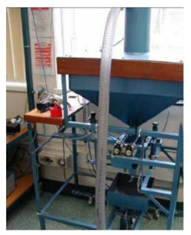
Figure 3: Sand-weighing machine (e-Laboratory Hardware).
