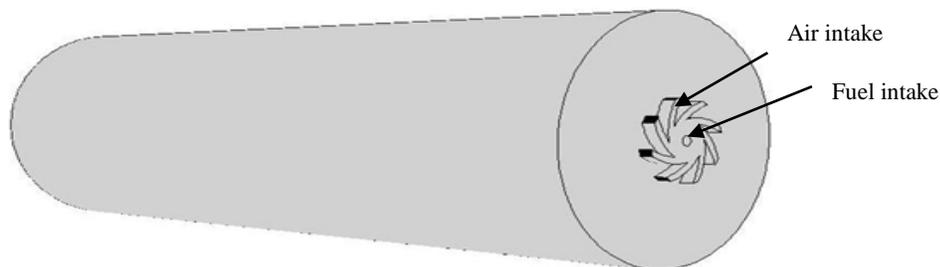
Figure 2 Combustor model
