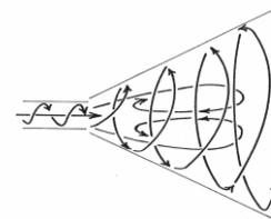
**Figure 1** Jet flow of high degree of swirl ( $S > 0.6$ ) resulting in significant lateral as well as longitudinal pressure gradients. Compared to its non-swirling counterpart, the jet is much wider, slower and there exist a central toroidal recirculation zone [8]
