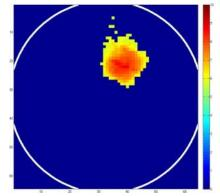
Figure 9 Gas model inserted with a diameter of 18.8 mm
