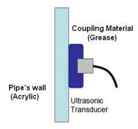
Figure 2 Acoustic coupling placement for ultrasound transmission
