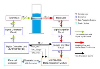
Figure 3 Electronics circuitry and the embedded system used in the Ultrasonic Tomography System
