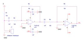
Figure 5 Signal conditioning circuit
