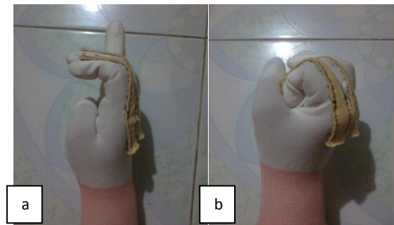
Fig. 5: Finger activities; (a) sensor#1 is half bend, sensor#2 is half bend (b) sensor#1 & sensor#2 are full bend.
