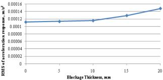
Fig. 6 RMS response at different blockage thicknesses
