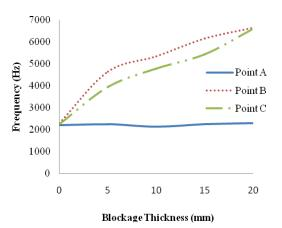
Fig. 5 Frequency response of different accelerometer locations
