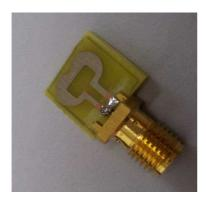
Figure 2. The prototype of the proposed antenna.
