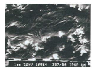
Fig. 3: SEM image of the pure PEO 600K membrane
