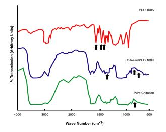
Fig. 10: IR spectra for PEO 100K, Chitosan-PEO 100K blend and pure Chitosan
