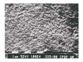
Fig. 6: SEM image of the chitosan-PEO 100K blend membrane
