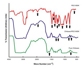
Fig. 9: IR spectra for PEO 600K, Chitosan-PEO 600K blend and pure Chitosan
