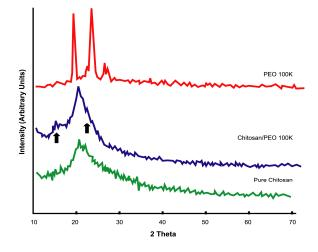
Fig. 8: X-ray diffractograms of pure PEO 100K, Chitosan-PEO 100K blend and pure Chitosan
