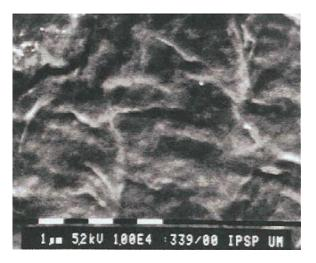
Fig. 5: SEM image of the chitosan-PEO 600K blend membrane
