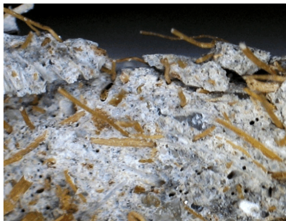
Fig. 24: Crack bridging and small holes observed in the fracture surface of composite cement reinforced with 9 wt. % of coconut fiber.
