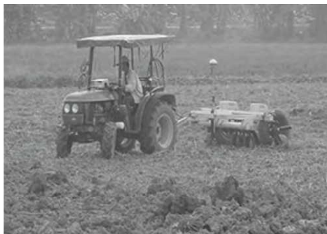
Figure 2: Soil ECa sensor integrated with Trimble Ag132 DGPS pulled by a tractor
