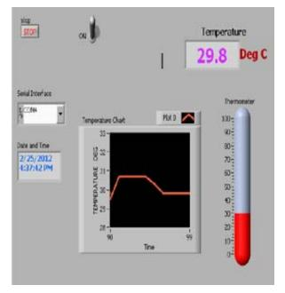
**Figure-7.** Front panel of the temperature data logging monitoring software for end users. The temperature in shown in Celsius (plot and numeric value) with the current date and time.
