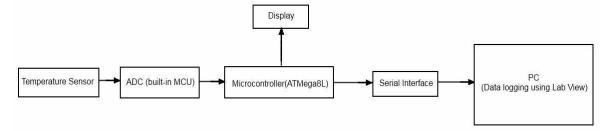
Figure-2. Block diagram of the temperature data logging system.
