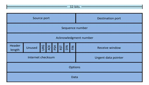
Figure 2.2: TCP segment structure
