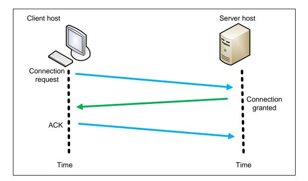
Figure 2.3: TCP connection establishment
