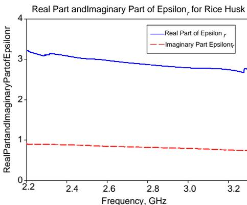
**Figure 1.** Real and imaginary parts of Epsilon<sub>r</sub> (dielectric constant) for rice husk.
