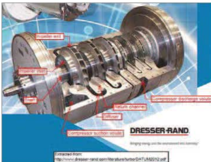
Fig. 2: Typical cross-sectional view of centrifugal compressor [6]
