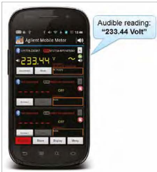
Figure 2: Android smartphone provides audible reading on multimeter's measurement for greater safety
