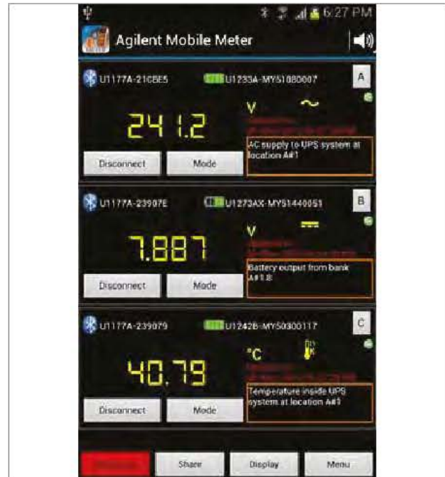
Figure 3: Wirelessly monitor 3 handheld meters' measurements using free Agilent Mobile Meter apps
