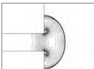
(iii) Shock front position at x = 13.75 \text{ cm} , density contours step 0.01
