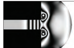
(vii) Shock front position at x = 33.5 \text{ cm} , density fringes step 0.1
