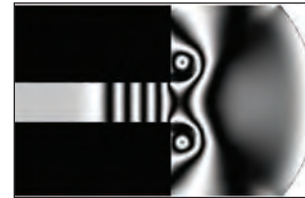
(viii) Shock front position at x = 38.5 \text{ cm} , density fringes step 0.1
