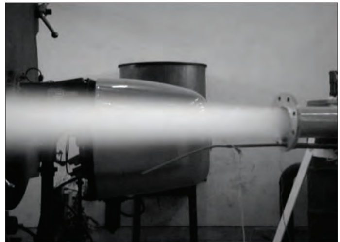
Figure 2: Photograph of post-shocked high speed air delivered from end section of the shock tube
