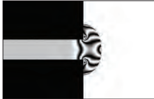
(ii) Shock front position at x = 9.0 \text{ cm} , density fringes step 0.1
