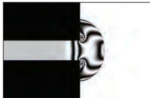
(iii) Shock front position at x = 13.75 \text{ cm} , density fringes step 0.1
