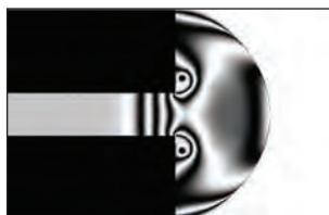
(v) Shock front position at x = 23.5 \text{ cm} , density fringes step 0.1
