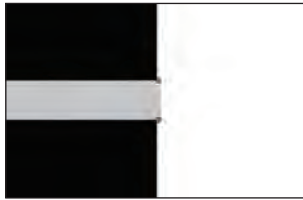
(i) Near end section of the shock tube, x = 0.0 \text{ cm} , density fringes step 0.1
