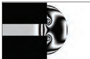
(iv) Shock front position at x = 18.5 \text{ cm} , density fringes step 0.1
