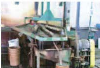
The shaking table used to collect gold nuggets or coarse gold particles
