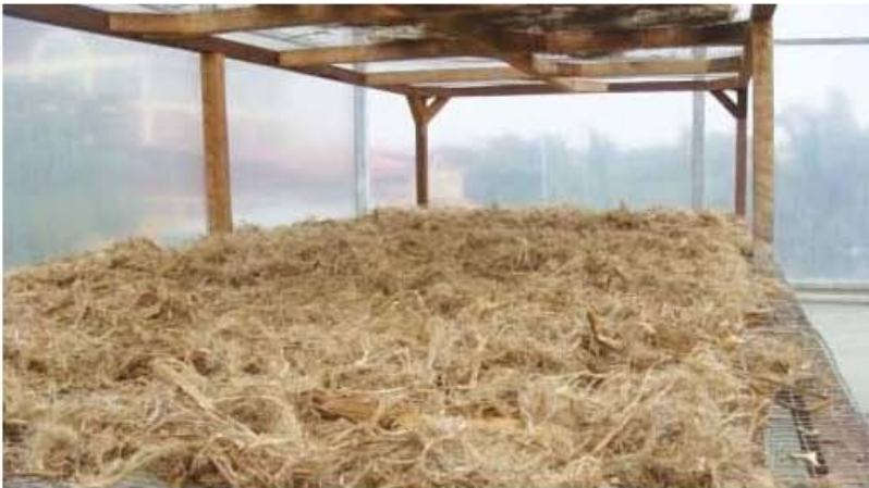
Figure 4: Drying process of pineapple leaf fibre in a solar drying house
