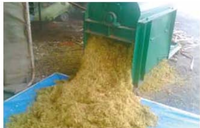
Figure 3: Mechanical extraction of pineapple leaf fibre using kenaf decorticator
