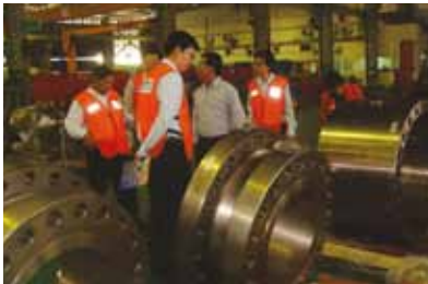
Valve closures ready to be assembled at the shop floor
