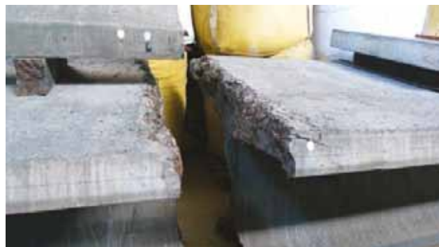
Figure 1: High strength ductile concrete loaded to failure
