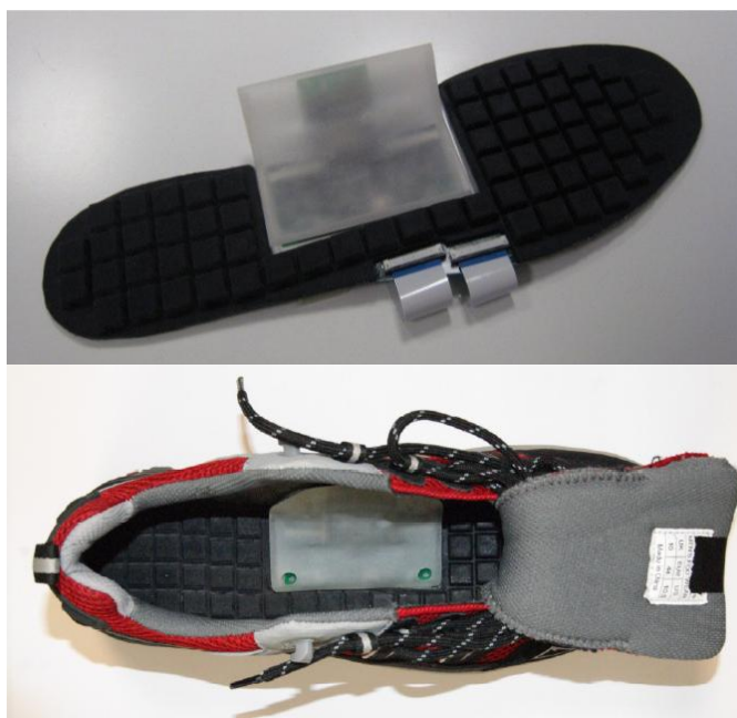
Figure 35. De Rossi et al. insole sensor system and the system fitted inside a shoe.
