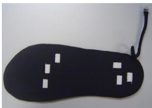
Figure 24. Fabric pressure sensing array indicating sensor placement [30].
