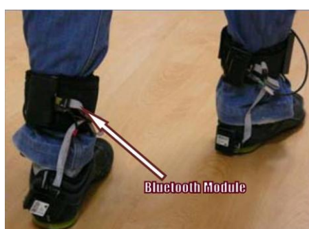
Figure 22. A wireless systems for gait and posture analysis based on pressure insoles and inertial measurement units [52].
