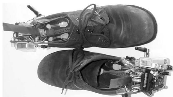
Figure 22. A wireless systems for gait and posture analysis based on pressure insoles and inertial measurement units [52].
