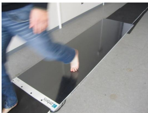
Figure 2. A platform based foot plantar pressure sensor by Zebris Medical GmbH [25].
