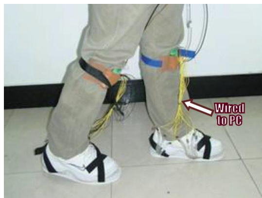
Figure 17. Biometric identification based on foot pressure pattern changes. Modified from [6].
