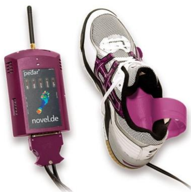
Figure 3. An in-shoe based foot plantar pressure sensor by Pedar ® Novel [24].
