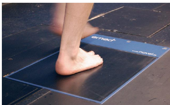
Figure 2. A platform based foot plantar pressure sensor by Zebris Medical GmbH [25].
