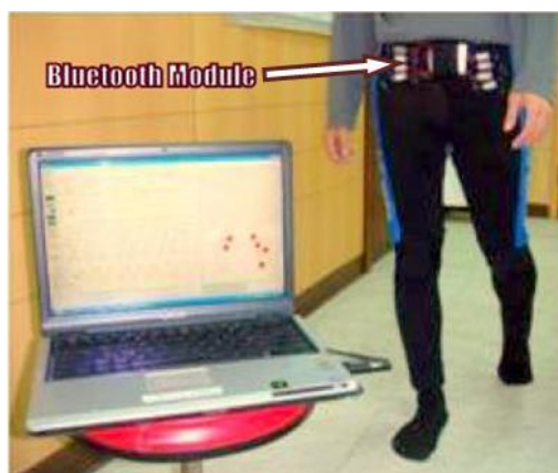
Figure 23. A wireless gait analysis system by digital textile sensors [53].
