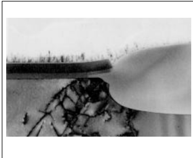
Figure 2.7: Stress damage in silicon substrate [7].
