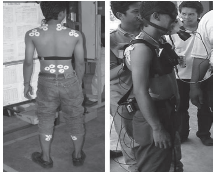
Figure 1. Selected muscles were attached with Ag-AgCl electrodes: deltoid-medial part (shoulder region); trapezius muscle (neck region); erector spinae (lower back), gastrocnemius muscle (leg region). An operator is equipped with a chest-mounted light-weight oxygen analyzer on his body to measure oxygen consumption (right).
