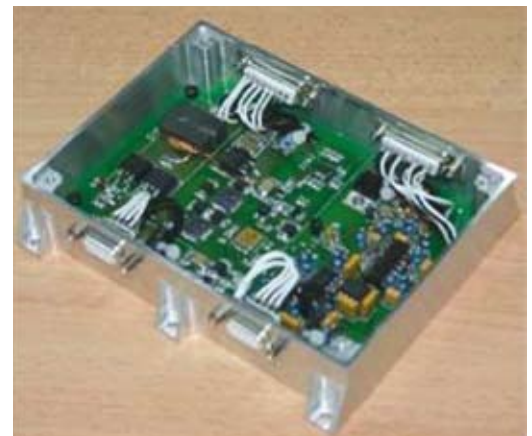
Figure 4: Battery charge regulator
