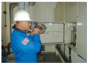
Thermographic monitoring of 415V switchgear reveals hotspots due to loose connections
