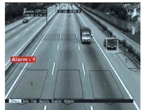
AID cameras detect incidents and are confirmed by CCTVs
