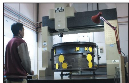
An engineer works on the highly-precise co-ordinate measurement machine (CMM)
