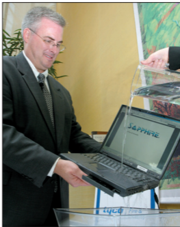
NOVEC fire protection liquid poured over a laptop without causing damage to the computer equipment.
