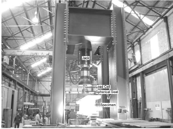
Figure 4: Specimen SB3 in testing frame (heavy structural laboratory of School of Civil and Environmental Engineering - University of New South Wales, Sydney, Australia)
