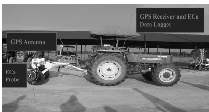
Figure 2: A GPS mounted on Veris 3100 unit attached to a tractor set for soil ECa survey at MARDI Seberang Prai
