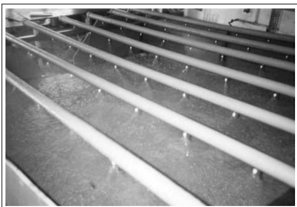
Plate 2: Runoff basin with bare clayey loam soil surface
