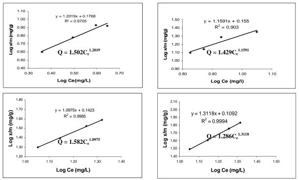
**Figure 1**. Freundlich Isotherm for Methylene Blue at (a) 10 ppm, (b) 25 ppm, (c) 50 ppm, (d) 75 ppm
