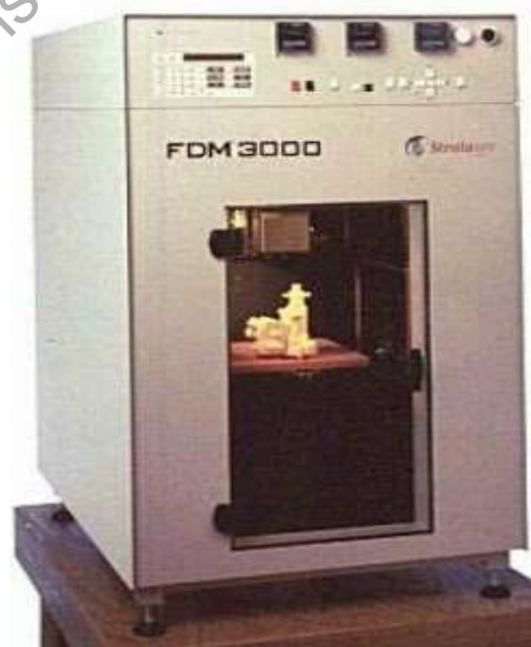
Figure 2.4: FDM 3000 machine (" http://www.stratasys.com/ ").
