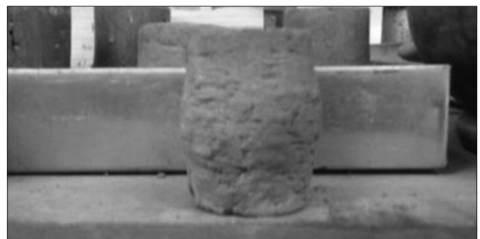
Figure 2: Specimen upon completion of triaxial test
