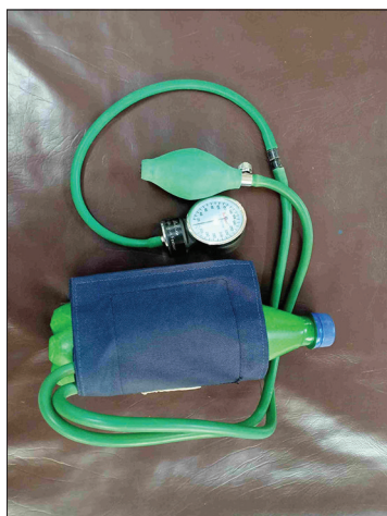
Figure 2: The modified sphygmomanometer apparatus for measuring isometric quadriceps pressure difference
