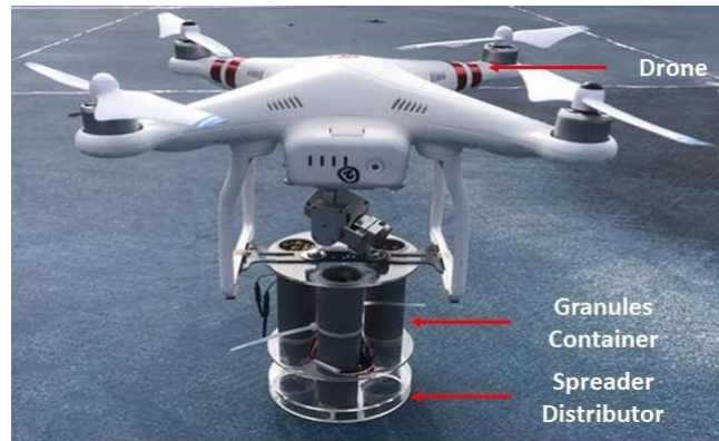
Figure 5. Drone along with container granules distributor.
