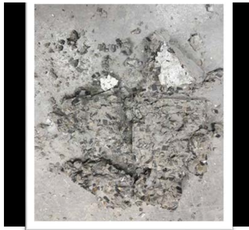
Figure 5. GPC20 after compressive strength testing.
