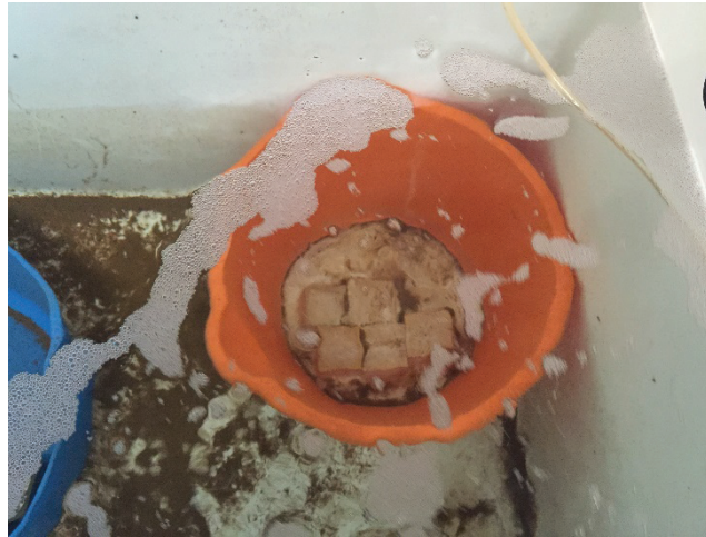
FIGURE 1. Immersion of metakaolin geopolymers in seawater.
