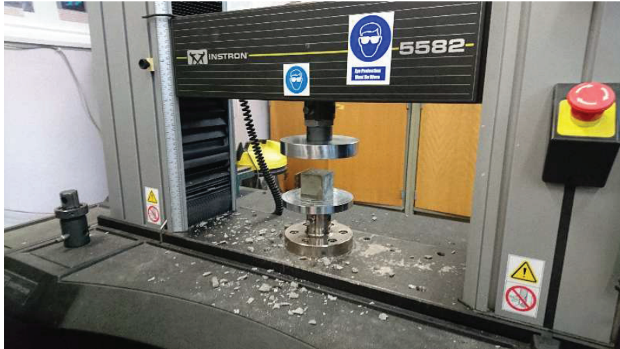
FIGURE 2. The set up for compressive strength testing.
