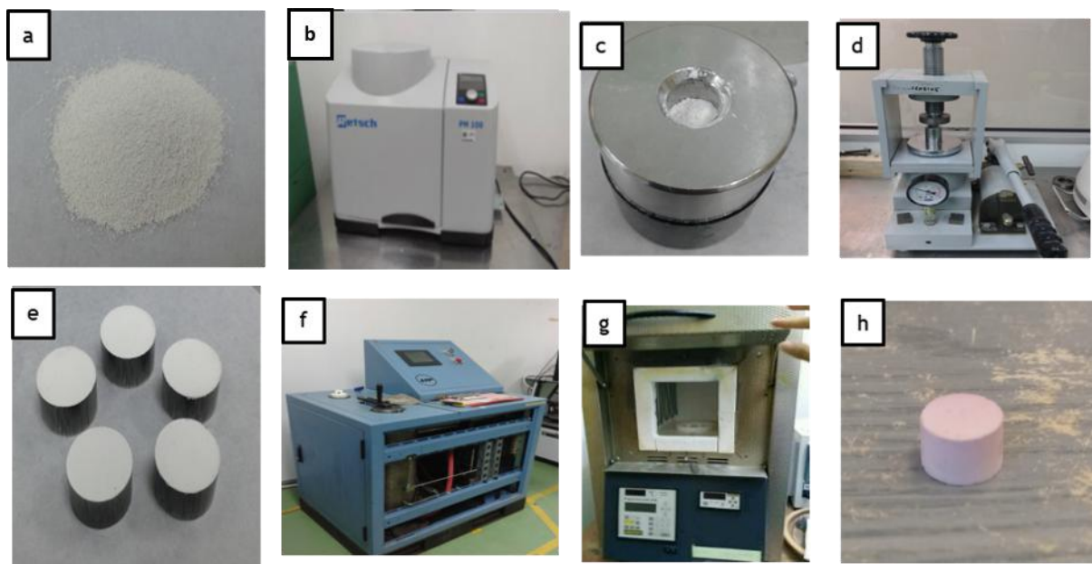
Figure 1. The procedure to fabricate \text{Al}_2\text{O}_3\text{-ZrO}_2 cutting tool (a) Preparing the powders (b) Blending in ball mill for 2 hours (c) Inserting powders into the mould (d) Pressing the mould by hydraulic hand press (e) Green body of ceramic compact (f) Pressing the powders by Cold Isostatic Press (g) Sintering the compacted powders (h) Finish product of ceramic cutting tool after sintering.
