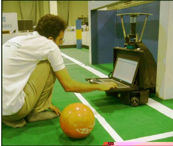
Fig. 1 Our robot is a 3-wheeled omni-directional mobile robot with an omni-directional vision system, a normal camera and a kicking device, and is controlled by a notebook PC.
