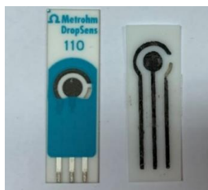
Figure 4. Photograph comparing DropSens 110 and homemade SPCE.
