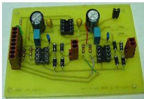
Figure 3: The smaller components mount on single-side PCB.
