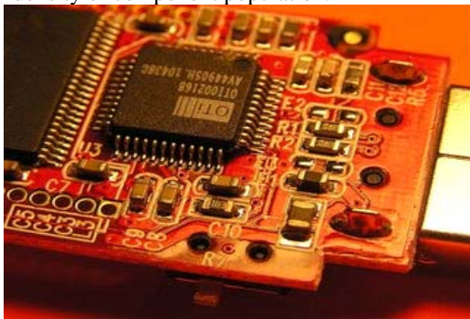
Figure 1: Surface-mount components on a keydrive's circuit board
