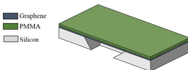
**Figure 1.** MEMS freestanding of PMMA/Graphene membrane.
