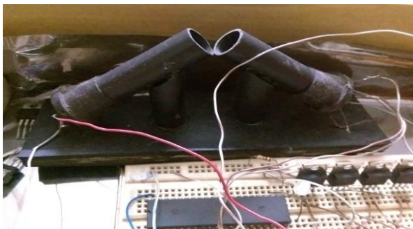
Fig. 9. Smoke detection Module (SDM)
