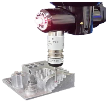
Fig. 3. Numerical control 3-D coordinate measuring machine (CMM)
