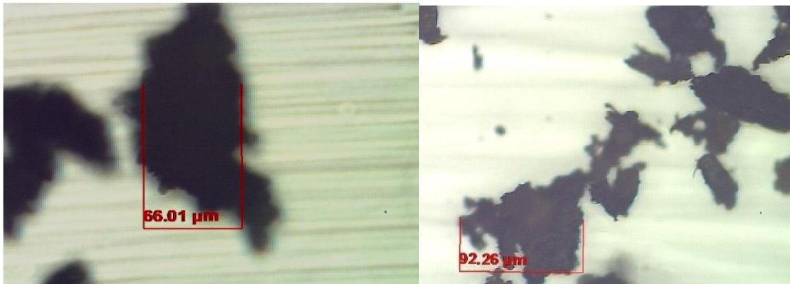
Figure 5. Micrograph of typical OPF dust in the samples obtained by Upright Microscope (20 ×).
