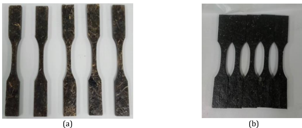
Figure 3. Tensile testing sample, a. OPF-Fiber composite and (b) OPF Powder composite.
