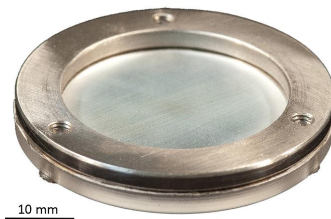
Figure 4. A macro photographic image showing a layer-by-layer triaxially aligned PVOH nanofibre construct.
