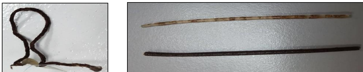
Figure 12. (Left) Flushed fibers after the degradation out of the extrusion die and (Right) the Successful extrusion of 5wt% Untreated PCSPC (bottom) and PCFC (top) composite filament.
